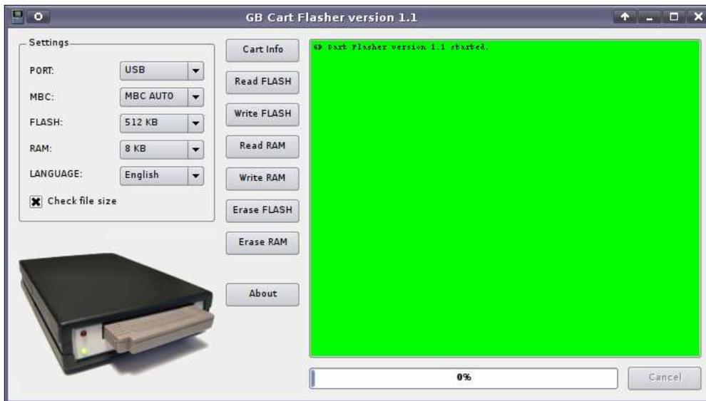
In *Settings* group you have to select appropriate Memory Bank Controller (MBC) which is installed in cartridge. If you do not know MBC type leave *MBC AUTO* setting. Select appropriate flash memory size and RAM memory size. Some memory sizes may be unavailable depending on MBC type selection. *Check file size* option allows writing files only with valid sizes when selected. If you want to check what is currently written to cartridge click *Cart Info* button:
